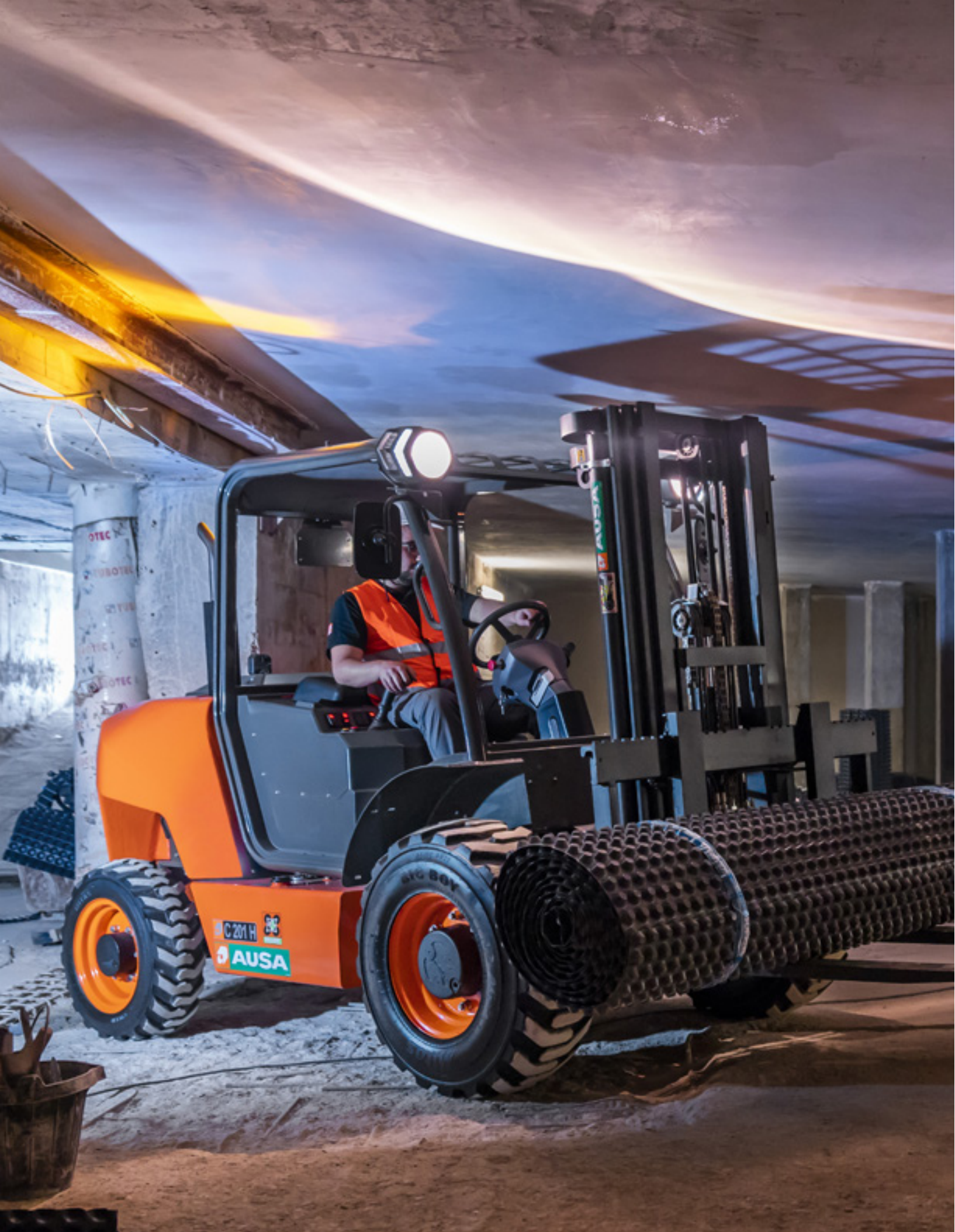
C201H 4,000 lb TRACTION 4x2 / 4x4 FULLGRIP® POWER 24.8 hp WIDTH 59.8 in TRANSMISSION HYDROSTATIC
