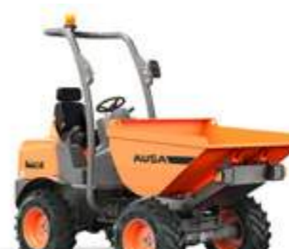
D150AHA 1500KG UNLOADING SYSTEM HIGH POWER 15.6KW WIDTH 1,480MM TRANSMISSION HYDROSTATIC
