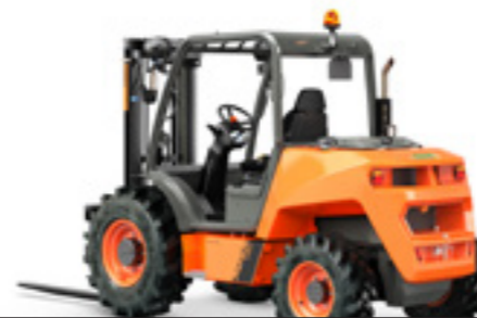
C251H 2500KG TRACTION 4x2 / 4x4 FULLGRIP® POWER 31.2KW WIDTH 1,520MM TRANSMISSION HYDROSTATIC
