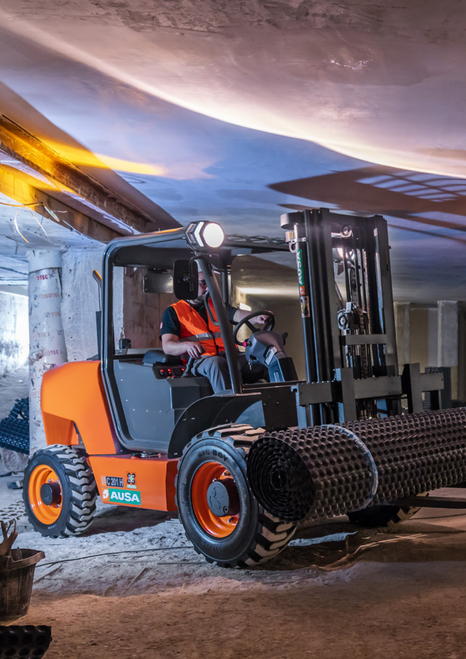
C201H 2000KG TRACTION 4x2 / 4x4 FULLGRIP® POWER 18.5KW WIDTH 1520MM TRANSMISSION HYDROSTATIC
