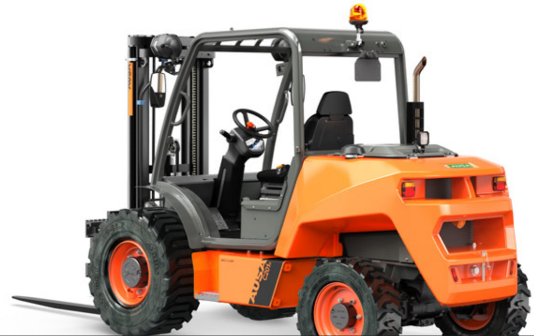
C201H 2000KG TRACTION 4x2 / 4x4 FULLGRIP® POWER 18.5KW WIDTH 1520MM TRANSMISSION HYDROSTATIC
