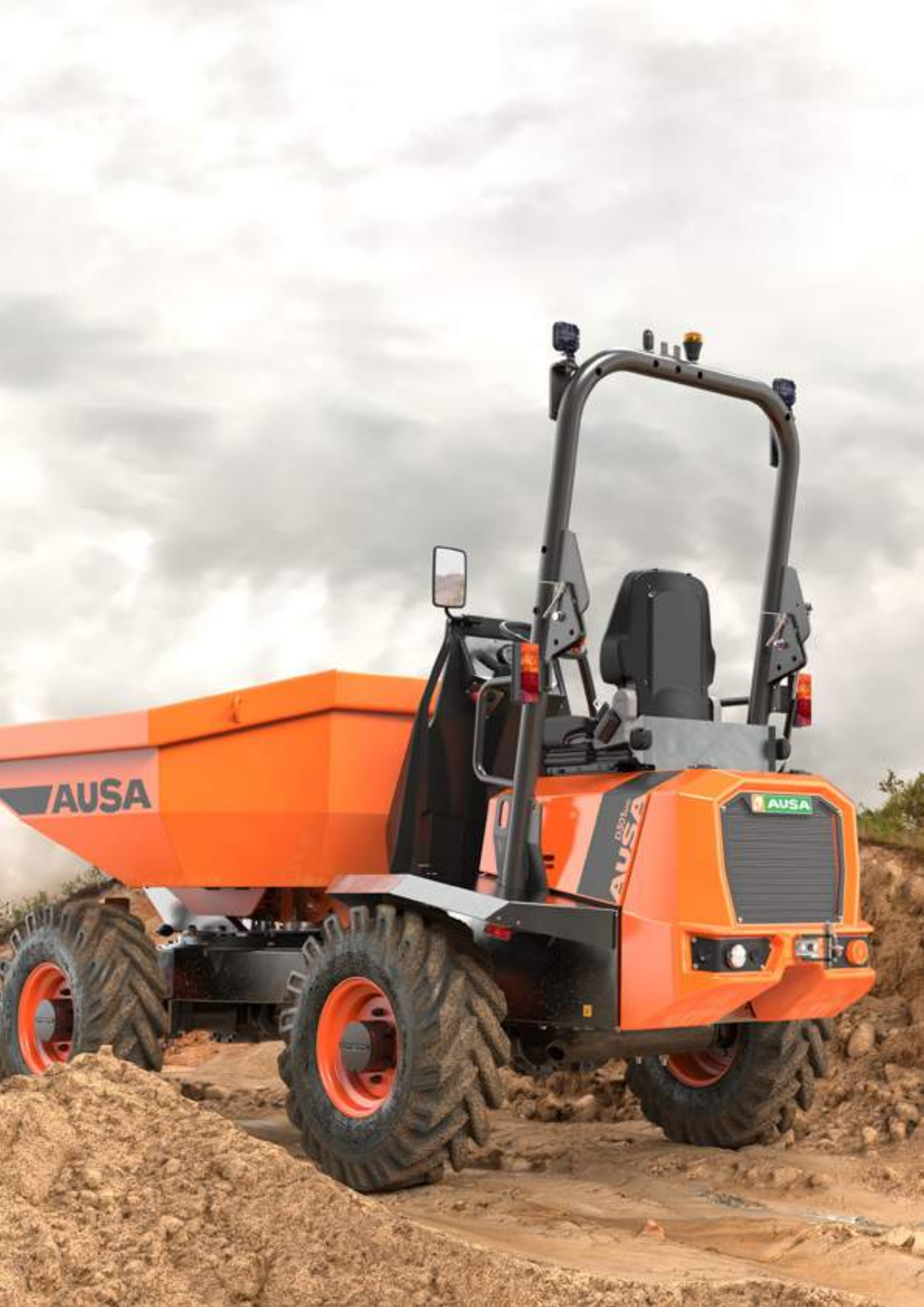
D201AHG 2000KG UNLOADING SYSTEM ROTATING POWER 18.5KW WIDTH 1,500MM TRANSMISSION HYDROSTATIC
