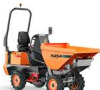
D101AEA COMPACT 1000KG UNLOADING SYSTEM HIGH POWER 19.6KW WIDTH 1,480MM TRANSMISSION ELECTRIC
