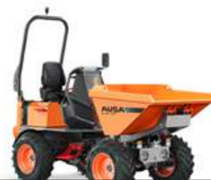
D151AEG 1500KG UNLOADING SYSTEM ROTATING POWER 19.6KW WIDTH 1,480MM TRANSMISSION ELECTRIC
