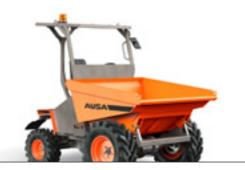
D150RM 1500KG UNLOADING SYSTEM FRONTAL TRACTION 4x2 POWER 12.1KW WIDTH 1,560MM TRANSMISSION MECHANICAL
