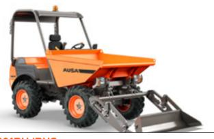
D201RH/RHS 2000KG UNLOADING SYSTEM FRONTAL TRACTION 4x4 POWER 18.5KW WIDTH 1,750MM TRANSMISSION HYDROSTATIC
