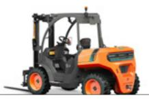
C151E 1500KG TRACTION 4x4 FULLGRIP® POWER 19.6KW WIDTH 1,390MM TRANSMISSION ELECTRIC
