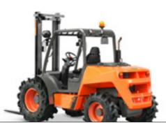
C351H 3500KG TRACTION 4x4 FULLGRIP® POWER 31.2KW WIDTH 1,780MM TRANSMISSION HYDROSTATIC
