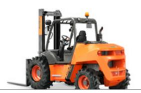
C501H 5000KG TRACTION 4x4 FULLGRIP® POWER 55KW WIDTH 2,010MM TRANSMISSION HYDROSTATIC
