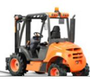
C150H 1500KG TRACTION 4x2 / 4x4 COMPEN® POWER 18.5KW WIDTH 1,300MM TRANSMISSION HYDROSTATIC
