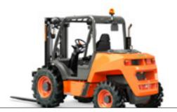
C251H 2500KG TRACTION 4x2 / 4x4 FULLGRIP® POWER 31.2KW WIDTH 1,520MM TRANSMISSION HYDROSTATIC
