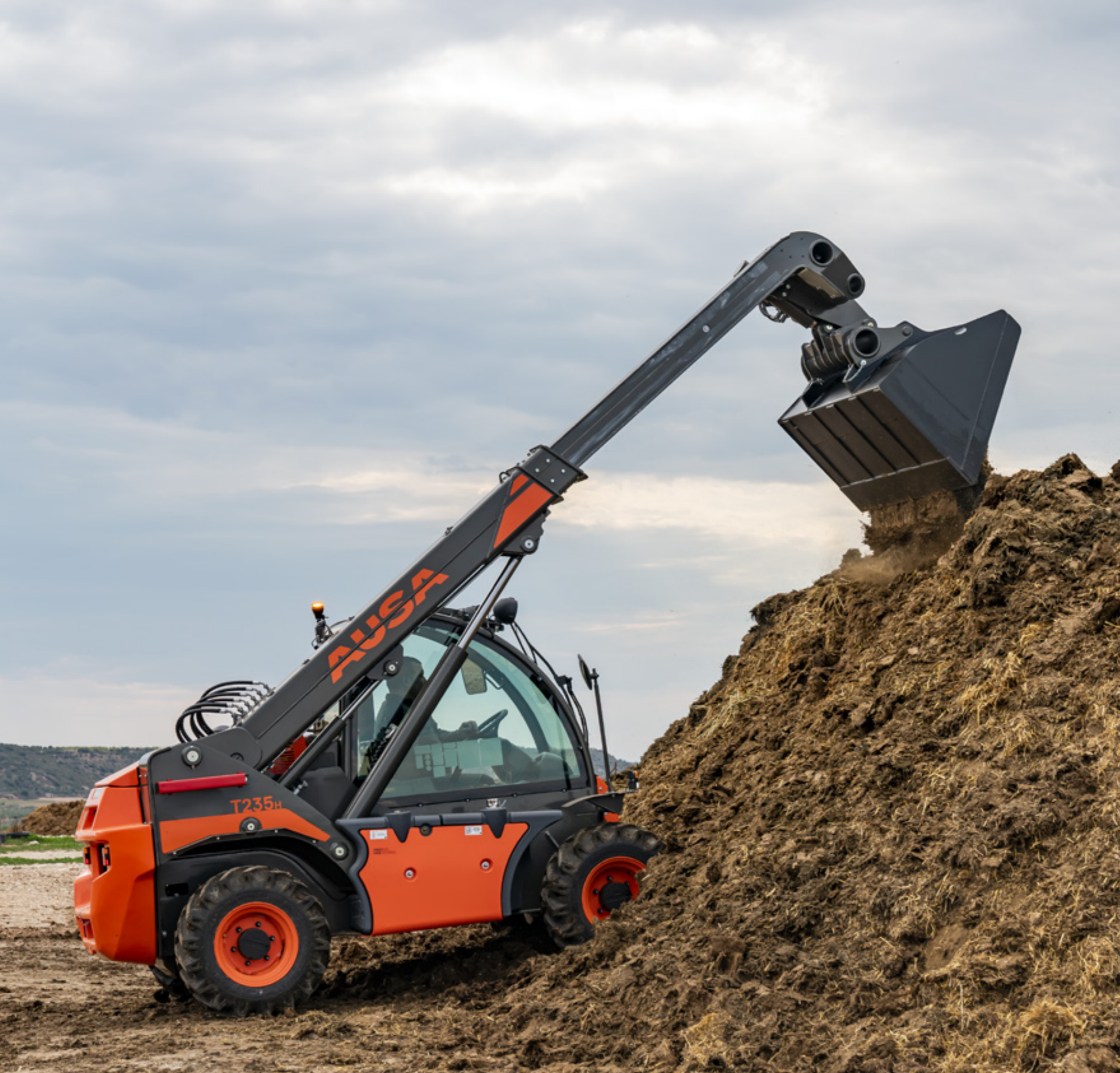
T204H 2000KG MAXIMUM LIFT 4,300MM POWER 32.8KW WIDTH 1,590MM TRANSMISSION HYDROSTATIC
