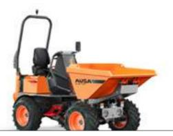
D151AEG 1500KG UNLOADING SYSTEM SWIVEL TIP POWER 19.6KW WIDTH 1,480MM TRANSMISSION ELECTRIC
