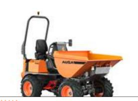
D151AHA 1500KG UNLOADING SYSTEM HIGH TIP POWER 15.4KW WIDTH 1,480MM TRANSMISSION HYDROSTATIC
