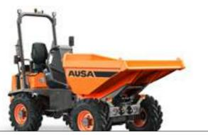
D301AHG 3000KG UNLOADING SYSTEM SWIVEL TIP POWER 18.5KW WIDTH 1,750MM TRANSMISSION HYDROSTATIC
