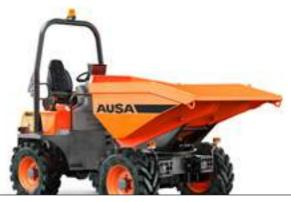
D450AHG 4500KG UNLOADING SYSTEM SWIVEL TIP POWER 32.8KW WIDTH 1,870MM TRANSMISSION HYDROSTATIC
