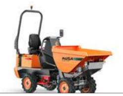
D101AEA COMPACT 1000KG UNLOADING SYSTEM HIGH TIP POWER 19.6KW WIDTH 1,000MM TRANSMISSION ELECTRIC
