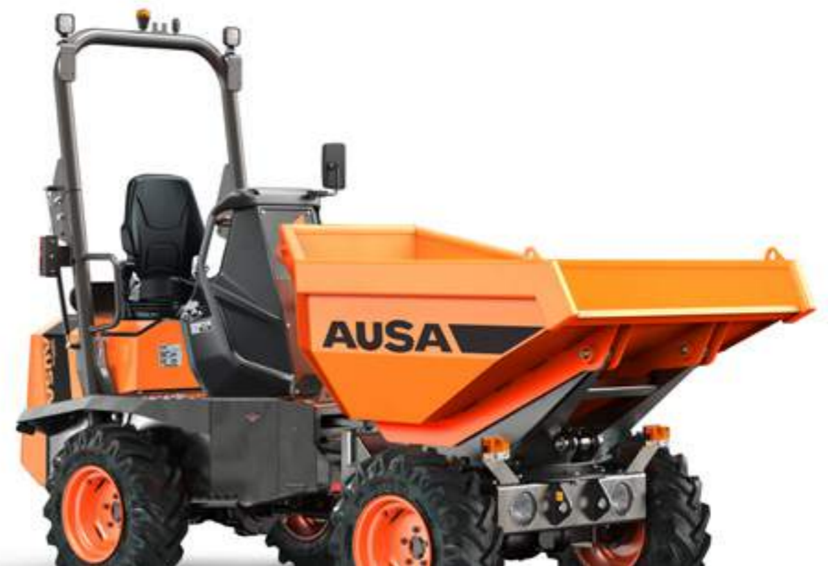
D201AHG 2000KG UNLOADING SYSTEM ROTATING POWER 18.5KW WIDTH 1,500MM TRANSMISSION HYDROSTATIC
