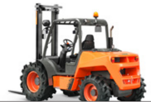
C351H 3500KG TRACTION 4x4 FULLGRIP® POWER 31.2KW WIDTH 1780MM TRANSMISSION HYDROSTATIC
