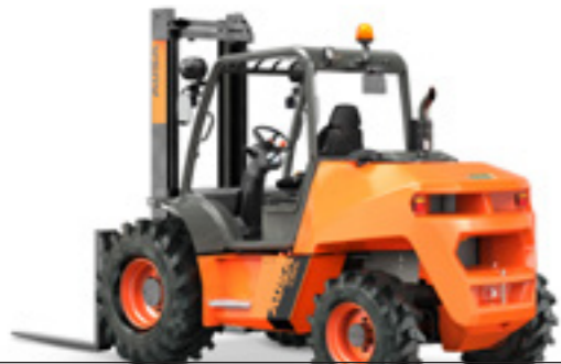
C501H 5000KG TRACTION 4x4 FULLGRIP® POWER 55KW WIDTH 2010MM TRANSMISSION HYDROSTATIC
