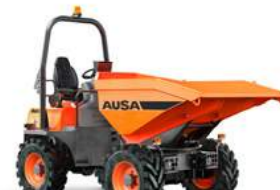
D450AHG 4500KG UNLOADING SYSTEM SWIVEL TIP POWER 32.8KW WIDTH 1,870MM TRANSMISSION HYDROSTATIC
