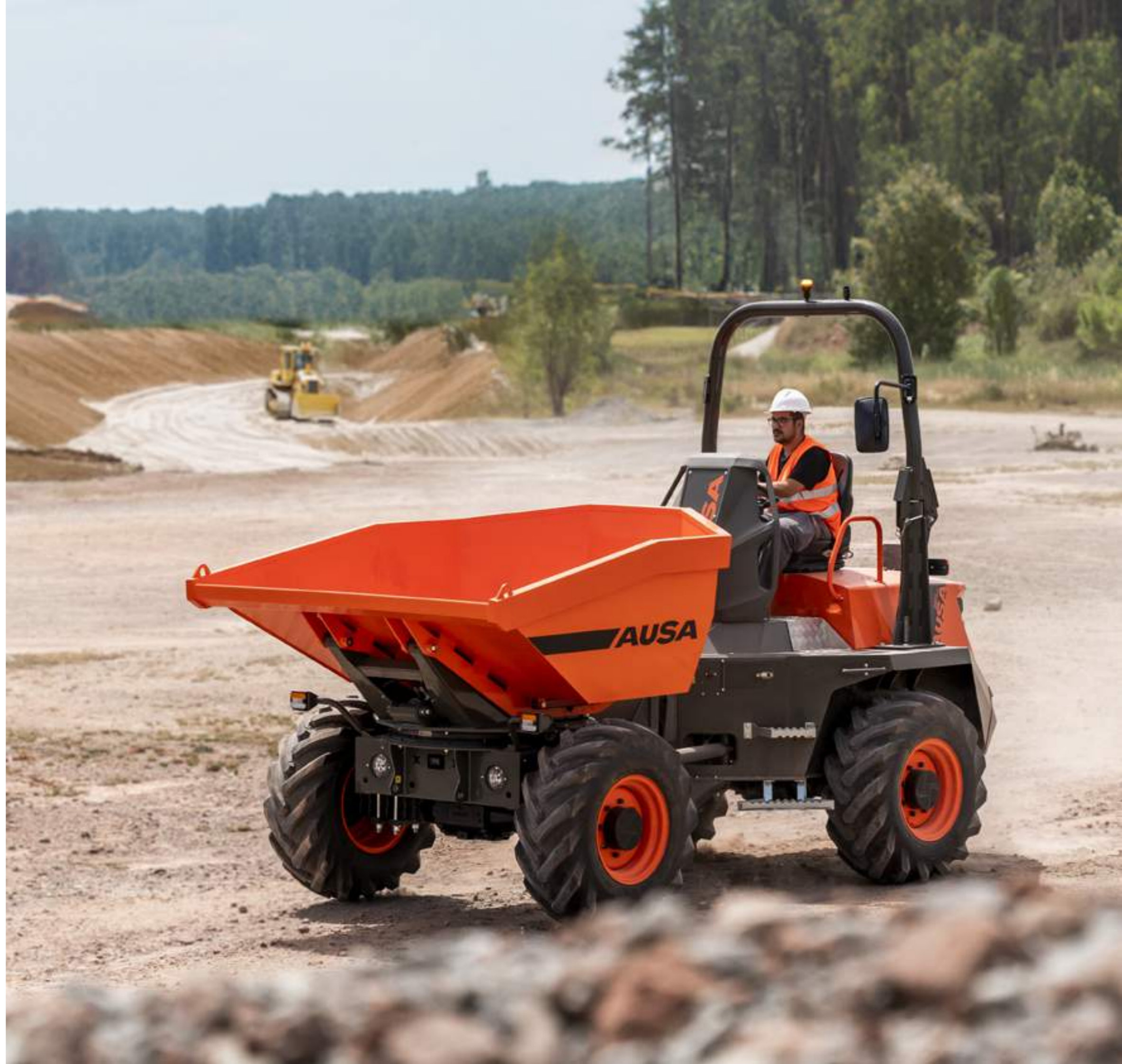
D1001APG 10000KG UNLOADING SYSTEM SWIVEL TIP POWER 55.4KW WIDTH 2,410MM TRANSMISSION TORQUE CONVERTER
