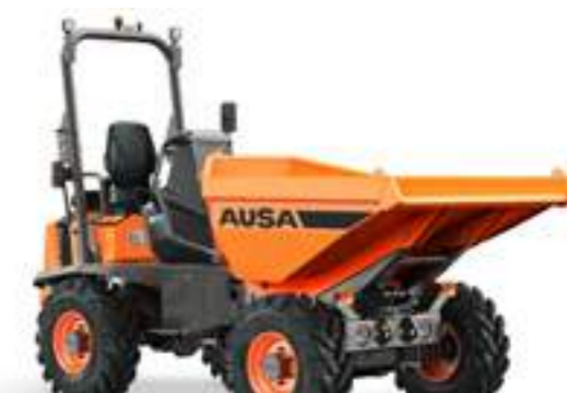
D301AHG 3000KG UNLOADING SYSTEM SWIVEL TIP POWER 18.5KW WIDTH 1,750MM TRANSMISSION HYDROSTATIC
