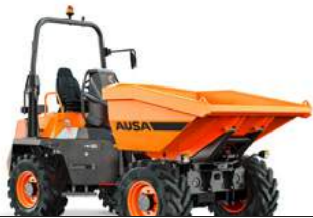
D601APG+ 6000KG UNLOADING SYSTEM SWIVEL TIP POWER 55.4KW WIDTH 2,210MM TRANSMISSION TORQUE CONVERTER
