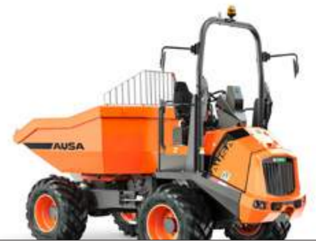
DR1001AHG 10000KG UNLOADING SYSTEM SWIVEL TIP POWER 55.4KW WIDTH 2,410MM TRANSMISSION HYDROSTATIC
