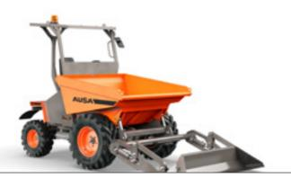
D175RMS 1750KG UNLOADING SYSTEM FRONTAL TRACTION 4x4 POWER 12.1KW WIDTH 1,560MM TRANSMISSION MECHANICAL
