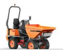
D101AHA 2,200 Ib UNLOADING SYSTEM HIGH TIP POWER 20.6 hp WIDTH 42.9 in TRANSMISSION HYDROSTATIC
