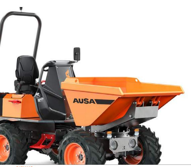
D151AHG 3,300 Ib UNLOADING SYSTEM SWIVEL TIP POWER 20.6 hp WIDTH 58.2 in TRANSMISSION HYDROSTATIC
