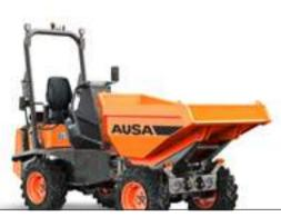
D201AHG 4,400 Ib UNLOADING SYSTEM ROTATING POWER 24.8 hp WIDTH 59 in TRANSMISSION HYDROSTATIC
