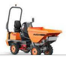
D101AHA COMPACT 2,200 Ib UNLOADING SYSTEM HIGH TIP POWER 20.6 hp WIDTH 39.4 in TRANSMISSION HYDROSTATIC
