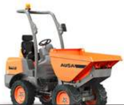
D100AHA 2,200 lb UNLOADING SYSTEM HIGH POWER 20.9 hp WIDTH 43.3 in TRANSMISSION HYDROSTATIC
