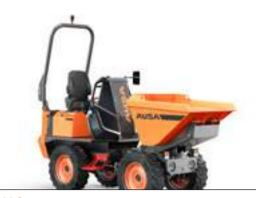
D101AHG 2,200 Ib UNLOADING SYSTEM SWIVEL TIP POWER 20.6 hp WIDTH 42.9 in TRANSMISSION HYDROSTATIC
