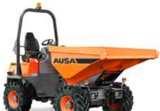
D350AHG 7,700 lb UNLOADING SYSTEM ROTATING POWER 44 hp WIDTH 72.8 in TRANSMISSION HYDROSTATIC
