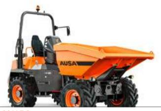
D601APG 13,200 Ib UNLOADING SYSTEM ROTATING POWER 74.3 hp WIDTH 87 in TRANSMISSION TORQUE CONVERTER
