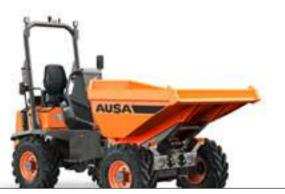
D301AHG 6,600 Ib UNLOADING SYSTEM ROTATING POWER 24.8 hp WIDTH 68.9 in TRANSMISSION HYDROSTATIC
