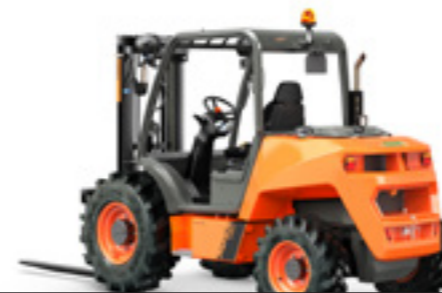
C251H 2500KG TRACTION 4x4 FULLGRIP® POWER 36.5KW WIDTH 1520MM TRANSMISSION HYDROSTATIC
