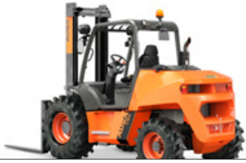
C401H 8,000 lb TRACTION 4x4 FULLGRIP® POWER 74 hp WIDTH 79.1 in TRANSMISSION HYDROSTATIC
