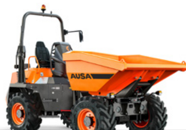
D601APG 13,200 lb UNLOADING SYSTEM ROTATING POWER 74.3 hp WIDTH 87 in TRANSMISSION TORQUE CONVERTER
