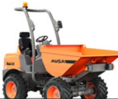
D150AHA 3,300 lb UNLOADING SYSTEM HIGH POWER 20.9 hp WIDTH 58.3 in TRANSMISSION HYDROSTATIC
