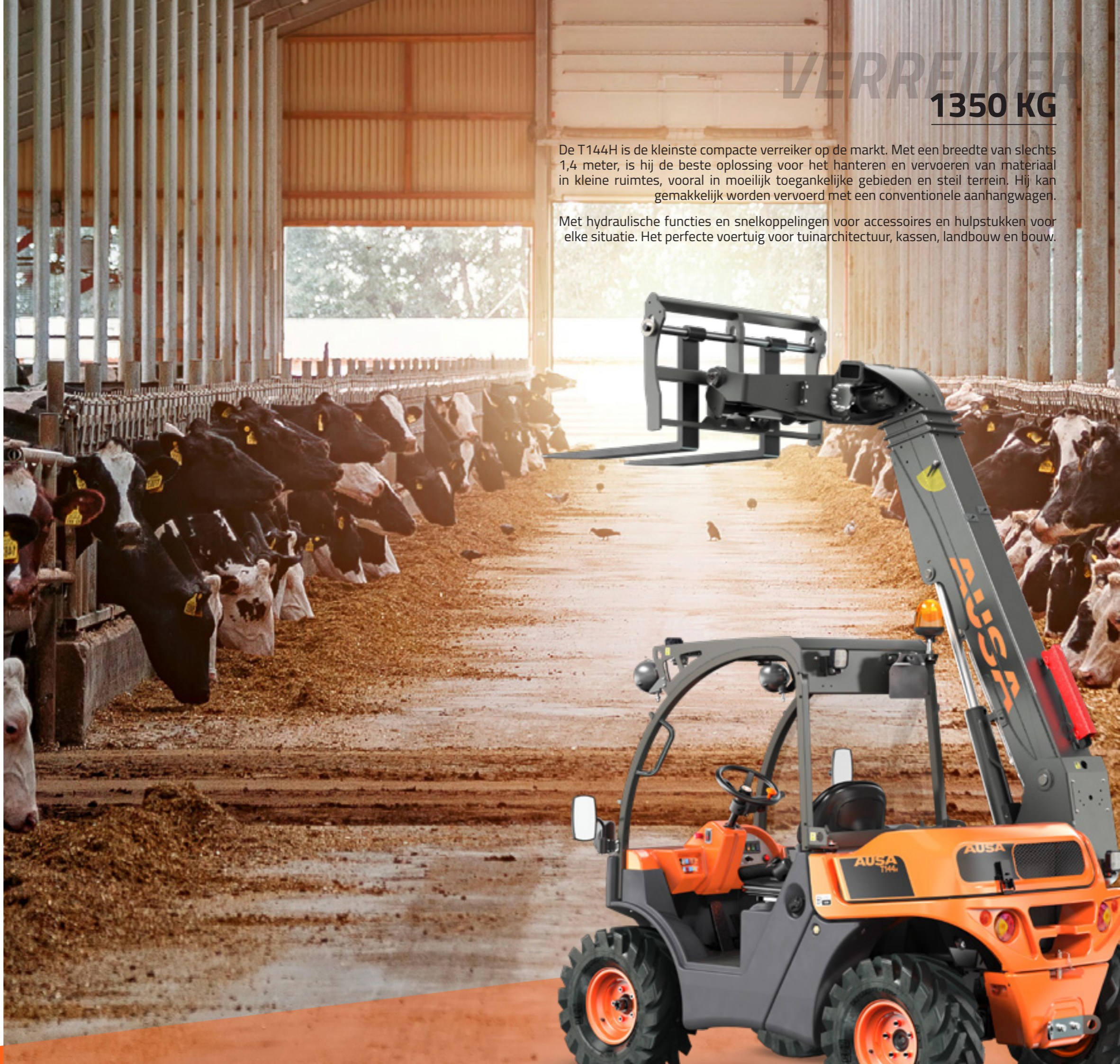
T144H 1350 KG MAXIMALE HEF 4,000MM VERMOGEN 18.5KW BREEDTE 1,405MM TRANSMISSIE HYDROSTATISCH
